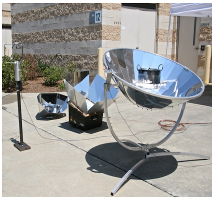
EPA testing: Sun Oven, Hot Pot and Sun Power solar cookers--all with zero emissions. Courtesy Jim Jetter. 2013
