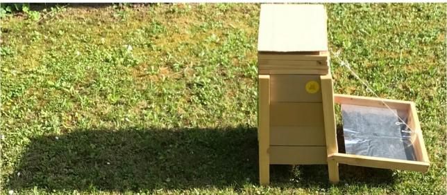
The picture above shows how to adjust the reflector once the sun is standing low above horizon: Low sun = low reflector = long shadow.
