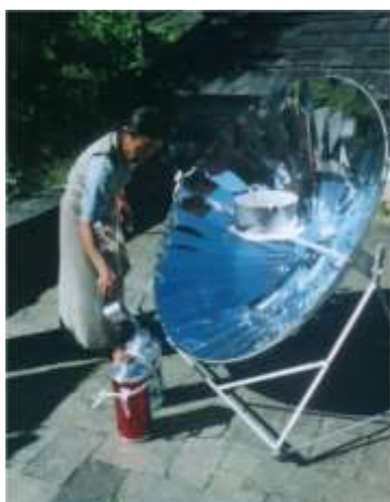
K. Schulte, Rotary Sveden: Project Nepal, Solar Cooker SK14 with thermos flascs
