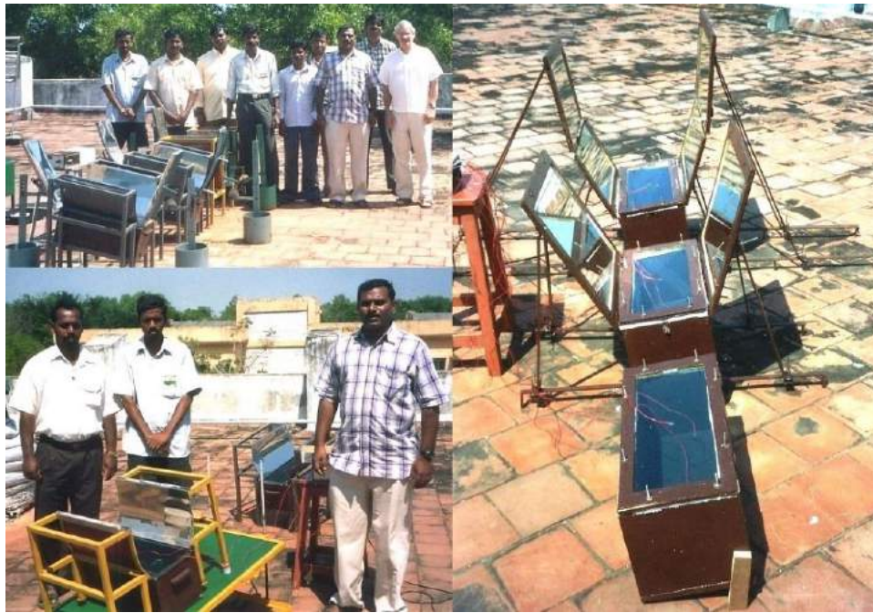
FIGURE 34. Compound Parabolic Concentrator (CPC) solar cooker study student engineering project at the Pondicherry Engineering College, south India in 2006, partly funded by the Foundation for World Education (FWE) (Rapaka, E. V. K., Report No.3: Study on the optical and thermal properties of a compound parabolic concentrator with and without end-wall reflectors for Pondicherry region , Oct. 9, 2006, Dept. of Mechanical Engineering, Pondicherry Engineering College, Pillaichavady, Pondicherry, India).
