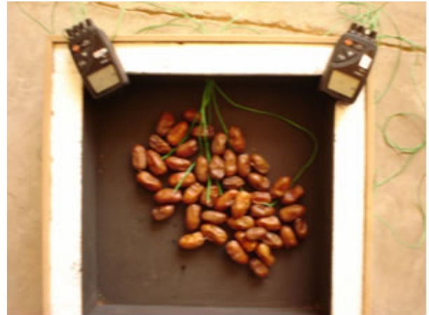
Fig. 1. Photo of the date fruits inside the flat solar collector
