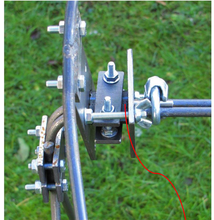
View of Friction Clutch at Axis with Bearing Plate, Pressure Plate and Friction Ring (22) with Friction Ring Holder (14)
