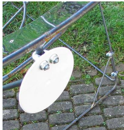
Shadow Indicator (22) connected to middle Ring Connector (8) with Rope Clamp (20)
