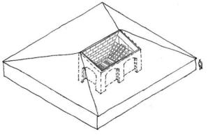
Thru-reflectorkitchen wall solar cooker with sloped hip roof building.
