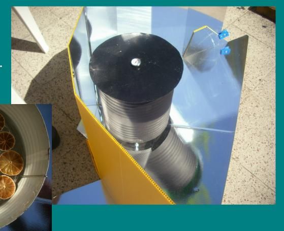
The Sun Rocket (left) is a small evacuated vacuum tube. It is a good device to pasteurize or boil water. In the meanwhile, food is prepared in the CooKit. More water is heated in the Jar-in-Jar heat trap simultaneously.
