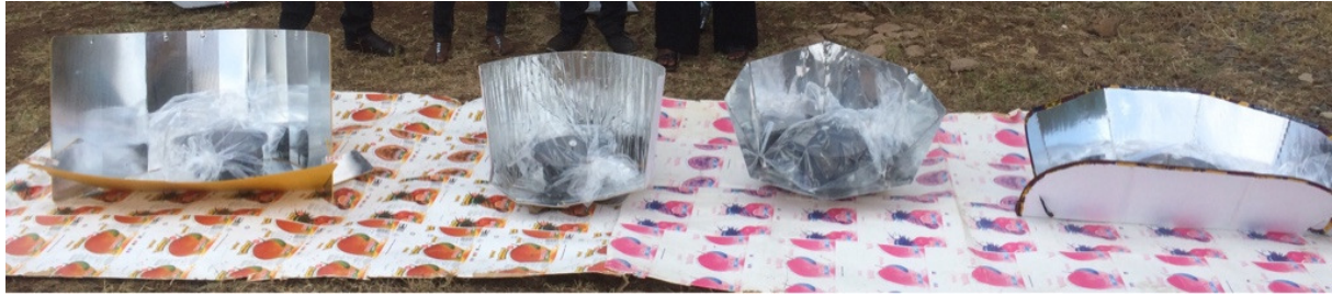
Die getesteten Kocher von links nach rechts: The tested cookers from left to right: LightOven III, Haines Foam Cooker, HotPot, CookIt
