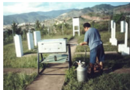
Fig. 4. Hybrid Solar Oven , with 110 VAC Electricity in Costa Rica (a, upper) and with LPG in Honduras (b, lower).
