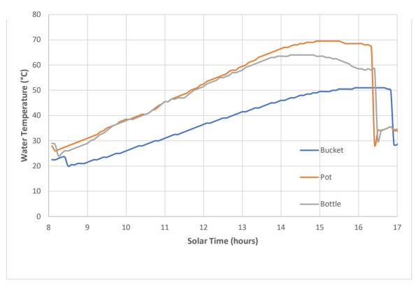
Temperatures achieved with several types of water containers in the Solar Household Energy Bank. The bottle is a 2-liter bottle, painted black, with the sensing element near the bottom of the bottle where the water is coolest.
