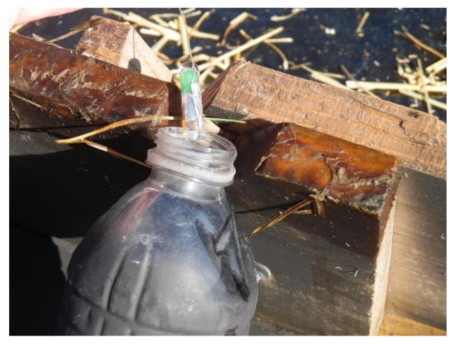
This shows a glass tube WAPI being removed from a water bottle at the end of the day. Since the green wax is still in the high end of the tube, pasteurization cannot be confirmed on this day.
