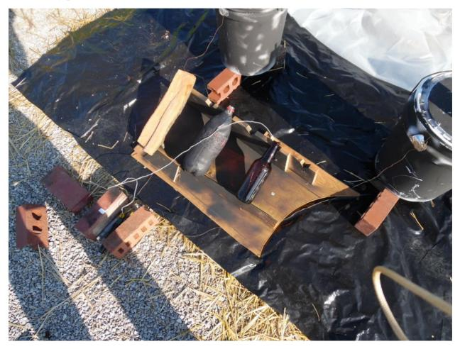
This photo shows two water bottles being pasteurized at the same time that wood is being dried and wash water if being heated. The bottles are a brown beer bottle and a plastic 2-liter bottle, painted
