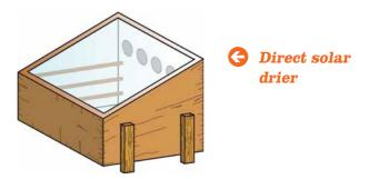
For the solar drier to operate most efficiently, the glass top must be at an angle of 45° to the sun, and the drier must be positioned to face south.
