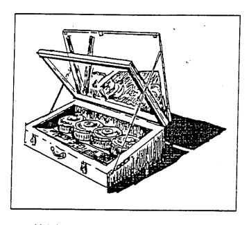
The external casing of the ovens is made from sheet steel. The frames for the liner and window are wooden. The inside of the oven is made from used newspaper printing plates (aluminium) which are purchased as scrap. The space between the liner and outer casing is insulated with about 50mm of mineral wool insulation. The box is rectangular in shape with a sloping
