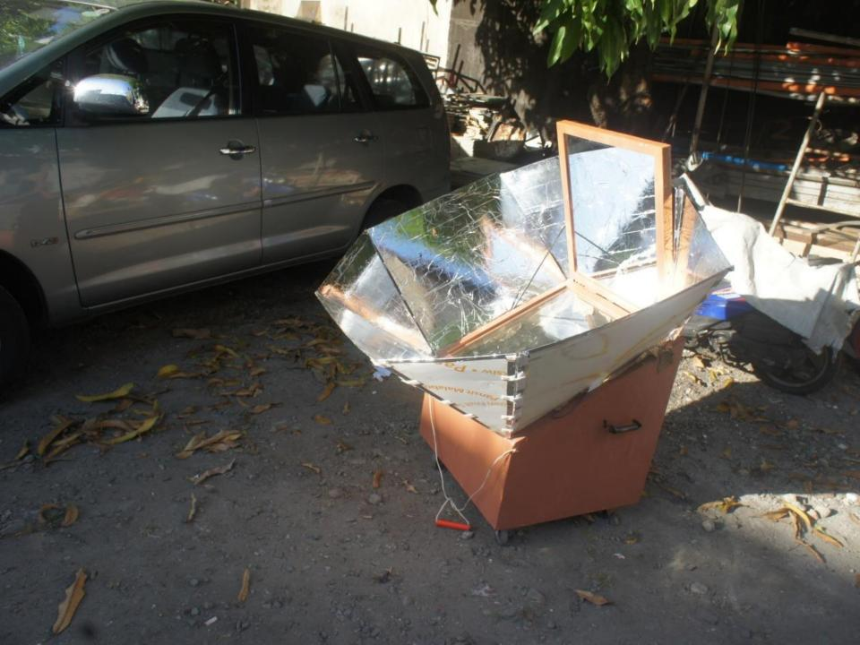
Gladly, after several trials, the oven gained 120 degrees Celsius at 9:00 in the morning and again on 2:30 in the afternoon. (No tests was conducted yet at noon time).
