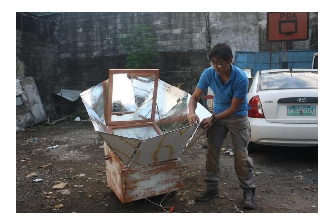
The used foam boards the thermal blanket and the velcro becoming the reflectors.
