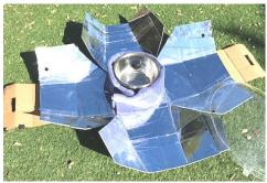
3. The petals form a square "basket" consisting of three layers of reflective foam insulation on each side. Before the "basket" is closed, towels or other
