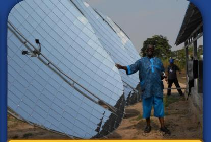
Large Scheffler parabolic reflectors provide fuel at a Cambodian commercial palm sugar processing center. Photo: Julie Greene, 2013
