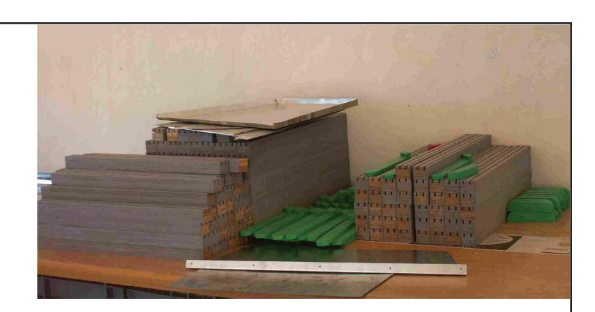
The manufacturing concept is aimed for serial production. Every step is standardized. As all work is supported by templates and jigs, measuring and marking are mostly obsolete.
