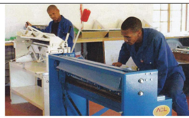
The cooker production requires a guillotine shear (left), a sheet metal bender (right), a circular saw and a hand-drill.
