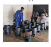
Wood-saving stoves and solar cookers are also being built in small series.
