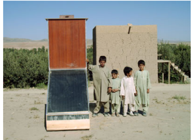
Picture 3: cupboard type solar dryer
