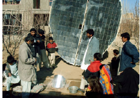
Picture 5: Scheffler Reflector at the Center for Renewable Energy in Bedmoschk. A traditional Tandor oven is heated with solar power.
