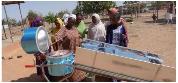
more fluid and a portion of the oil overflows into a special container. In the process, the heat transfers to metal cooking pots that are placed in the container. At peak operation, the vegetable oil can reach 200 °C (393 °F) or higher.
