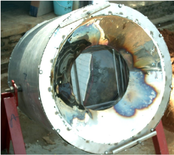
Fig. 7 total isolated iron block with heat resistant glas
