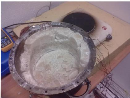
Prototype of storage solar cooker, developed by ITEA group at Universidad Carlos III de Madrid. After storing heat it is kept insulated with a prototype cover, 6 kg weight.
