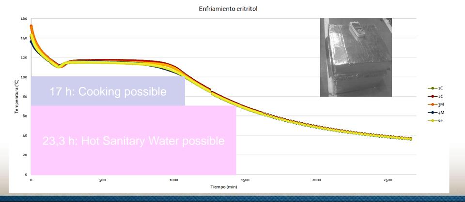
Prototype developed at Universidad Carlos III de Madrid, ITEA research group. Result: After storage, the utensil heats3 times 2 I of cold water (blue line), while the PCM cools down (grey and orange lines).
