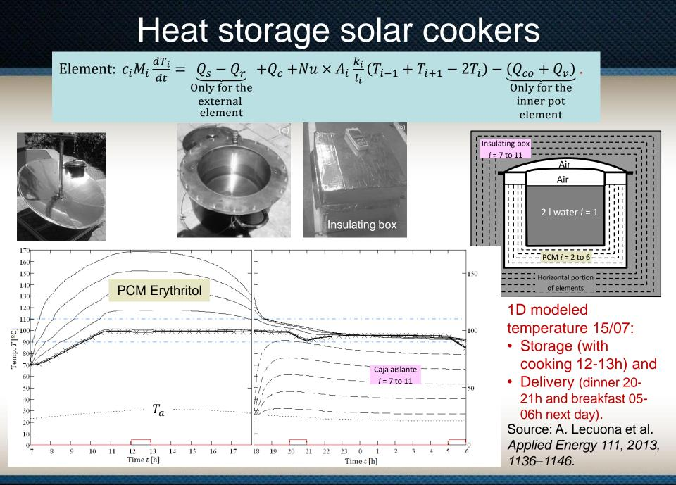
Prototype developed at Universidad Carlos III de Madrid, ITEA research group. Result: PCM temperature during heat retention with PCM initially completely melted. Testing result in the Master Thesis of Miriam Cabañas Martín (graduated with honors).
