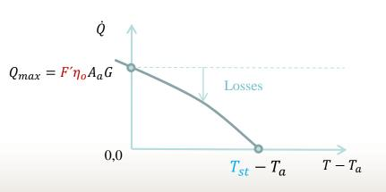
$$0 = C \frac{dT}{dt} = F' \left[ \underbrace{A_a G_T \eta_o}_{\text{Solar}} - \underbrace{AU(T_{st} - T_a)}_{\text{Pérdidas}} \right] \rightarrow AU_{st} = \frac{A_a G_T \eta_o}{T_{st} - T_a}$$
