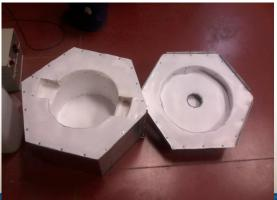
← Inner pot with flanges for joining with the outer pot.
