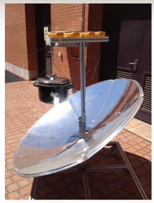
↑ Storing heat with a Chinese concentrating solar cooker. Cover for heat retention $\rightarrow$
