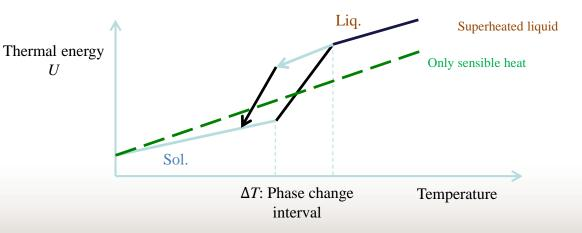
• Supercooling is a meta-stable process that reduces solidification temperature.
