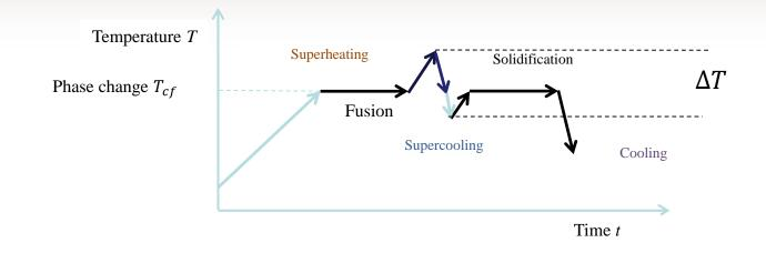
Modeling. Owing to the difficulty of the Stefan problem a temperature interval is assumed for phase change in the PCM (1D model):
