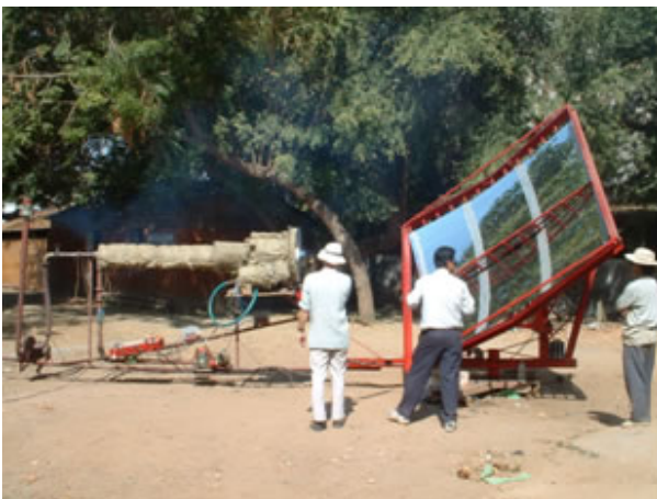
Fig.1 Experimental set-up for solar cremation in Baroda, India, with two axis tracking of the sun.
