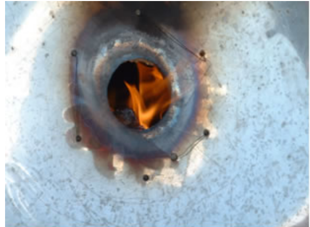
Fig.2 View into the glowing chamber during the final stages of the combustion. The focus was moved away to take the picture.
