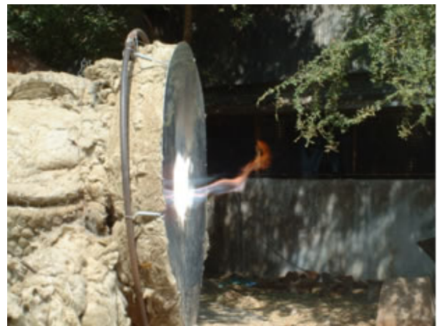
Fig.3 The flue gases are leaving the chamber through the focus opening and a long flame is seen, burning off without visible smoke.
