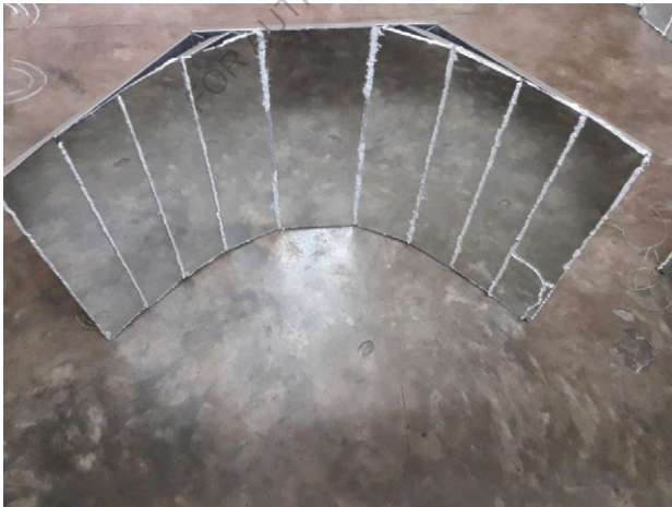
Fig-19 (9 segment reflector assembly)
