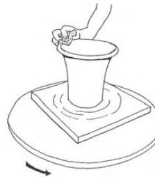
69. Sponge the rim, widening or narrowing the width as needed.
