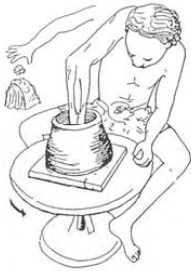
16. Remove excess clay from the inside bottom
