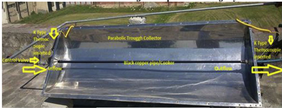
1.2: Experimental Setup of Parabolic trough collector
