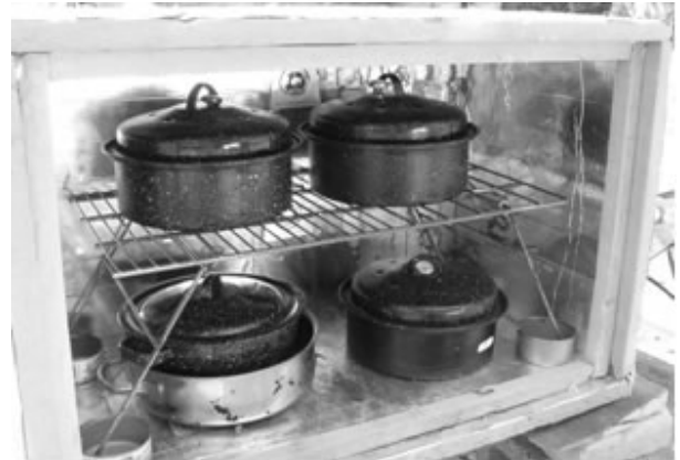
Fig.4 Sustained Heat Chamber. Three pots inside to be kept at cooking temperature. The lower left pot is in position on Hotplate to be brought up to cooking temperature.
