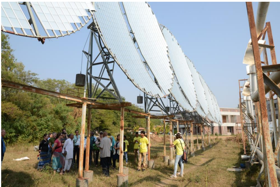
Industrial solar concentrators, Muni Seva Ashram, Gujarat, India. Photo: C. Cross 2017
