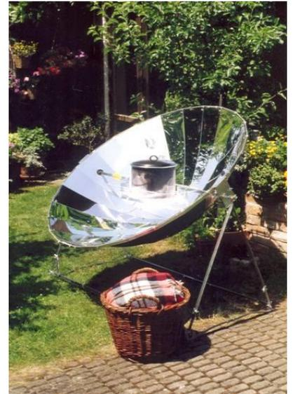
*Photo A3: Parabolic solar cooker with thermos basket*
