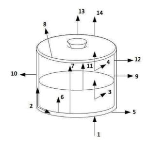
Heat energy movements in a cooking pot during the cooking process. Image courtesy by Ing. Verónica Frías, Mexico.
