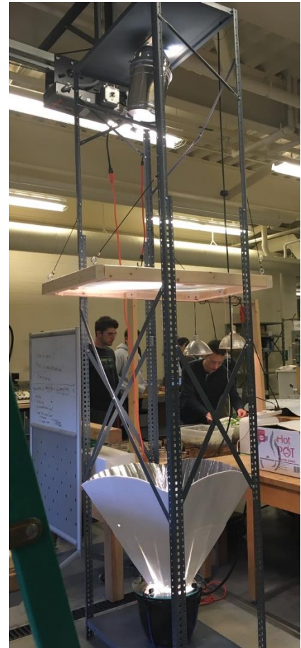
Solar simulator at Messiah College for testing solar cookers indoors. Photo Credit: Messiah College
