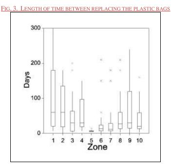
Fig. 3 shows a huge variation in the stated times with the shortest being very few days, and the longest being over a year. The duration of a heat resistant plastic bag used for solar cooking on a daily basis in other countries is approximately one month. The plastic bags are replaced by the refugee staff working in each zone, and the results show large zone-to-zone differences. In particular they show an apparent difference between zone 5 and the others.
